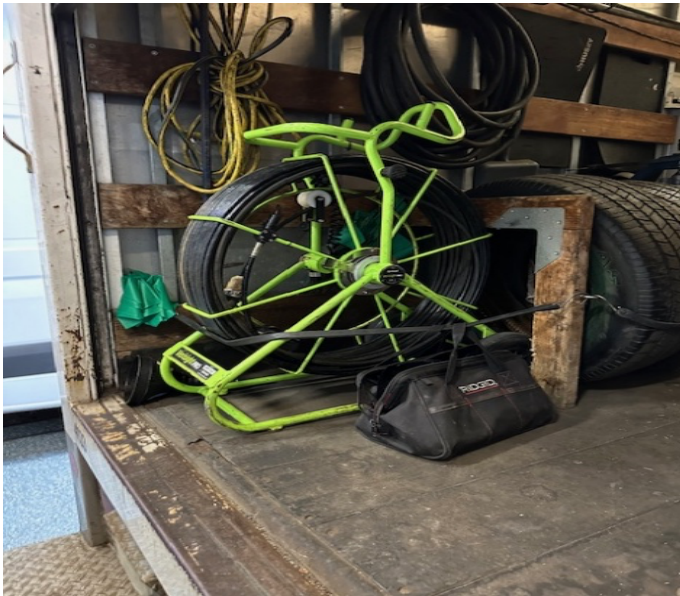
Photo 7: Inspection of of Daly City customer service truck equipped for providing lateral services as a courtesy to ratepayers including lateral jetter, push camera, and pipe locating equipment. Each customer that contacts the City for problems receives this service once and are informed of what the crew's findings are to help resolve problem.
